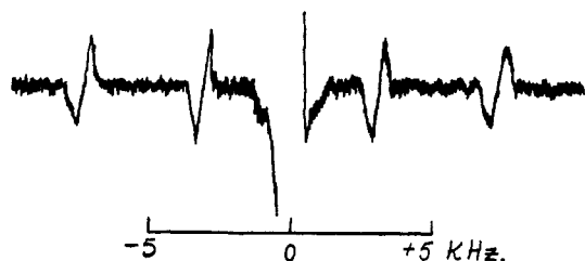
Figure 2. The deuterium magnetic resonance spectrum of lyotropic nematic phase d after separation of the bottom isotropic phase. The upper phase, which was studied, was a typical mobile nematic phase. The outer doublet is assigned to partially averaged nuclear quadrupole coupling in the deuterium atoms of the -\text{CD}_2- group and the inner doublet arises from the adjacent -\text{ND}_3^+ group. The deuterium signal of the \text{D}_2\text{O} was overmodulated at the center of the spectrum and has been omitted. The detection frequency was 4.1 MHz and the temperature 28^\circ .
